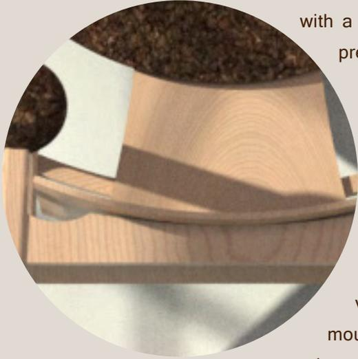
The backrest will be made by CNC cutting cross sections of Maple which will be glued together and covered in a veneer to give it the appearance of moulded plywood. This method will be used to ensure a strong and stable backrest.
