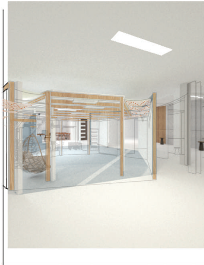
Timber frame structure with holding fabric. The installation included 4 acrylic plastic to hold the frame.
