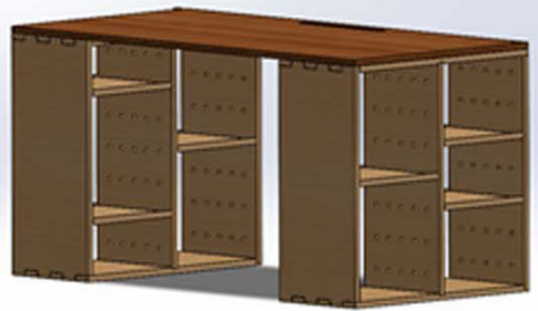
First CAD design with adjustable shelves and removable pins
