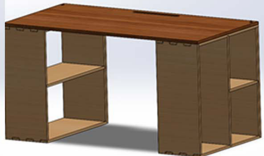
CAD designs with initial fixed pins design
